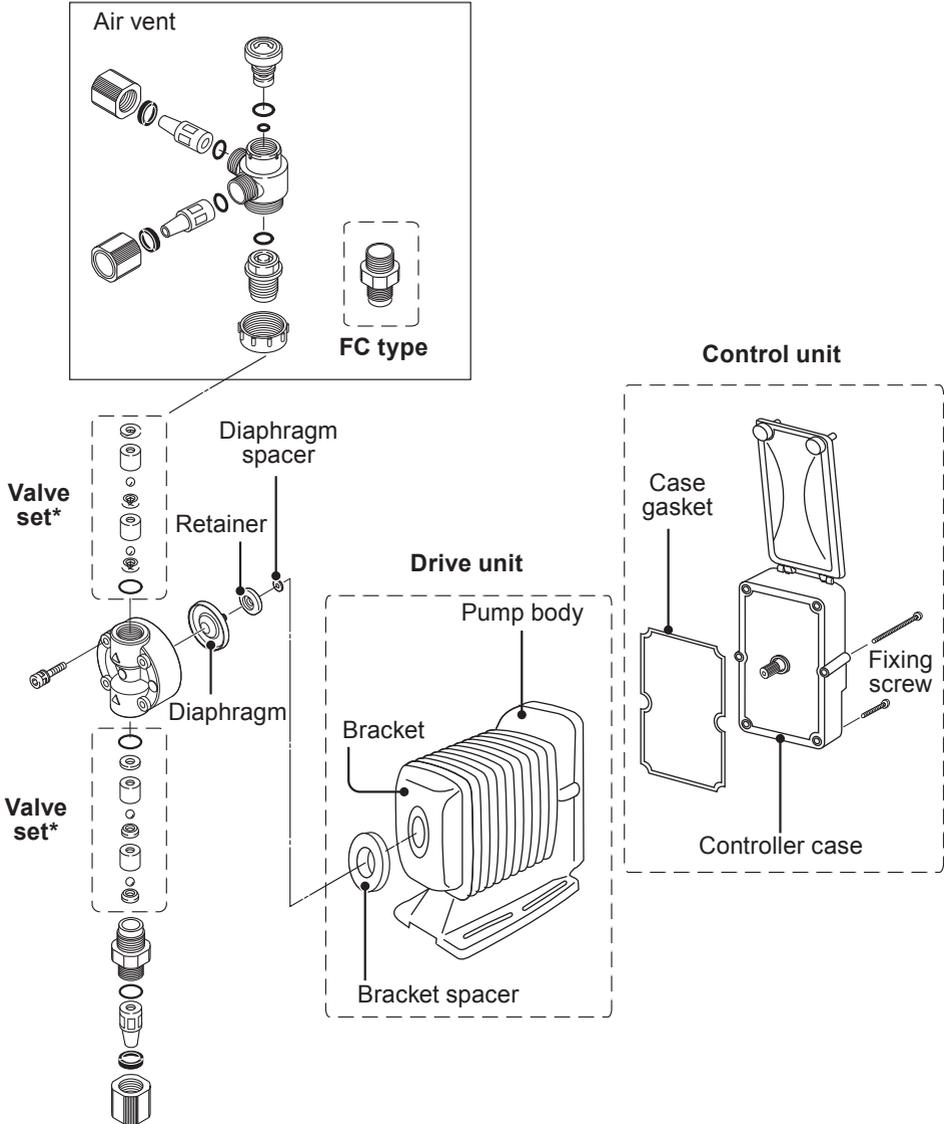
\*Wet end materials and their sizes differ with models. See "Valve set replacement" on page 81 for detail.
