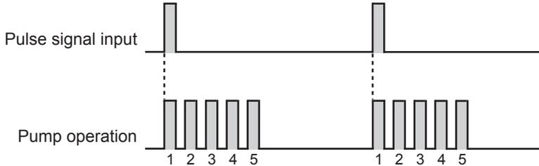
A buffer works when the pump receives the external signal before the programmed shots per signal is completed.
