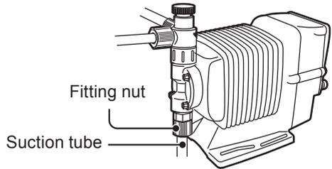
**2 Remove the fitting by an adjustable wrench or a spanner.**
