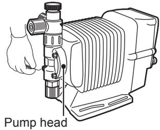
**4** Rotate and remove the diaphragm from the plunger (pump shaft).
