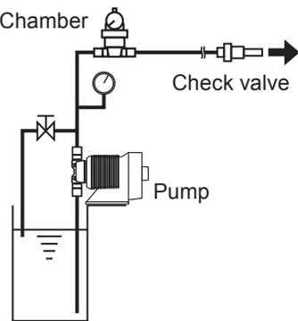
\*Flooded suction is recommended when handling a gaseous liquid such as sodium hypochlorite.
