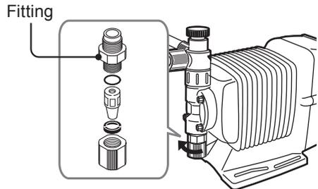
**3** Pull out the valve set by a pair of tweezers.
