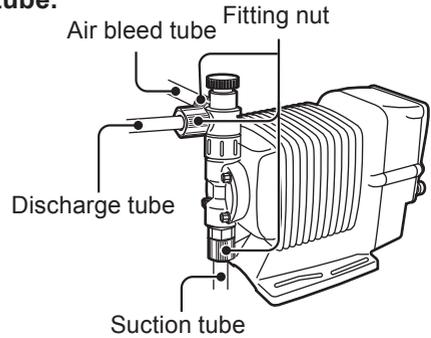
**3** Remove the pump head by a hexagon wrench.
