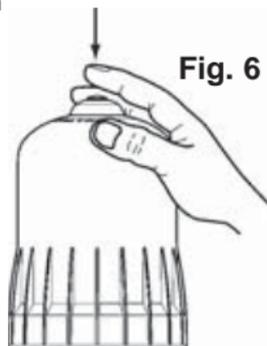
**NOTE:** The time required to prime the suction tube depends on the water flow-rate, the ratio setting and the length of the suction tube. To bleed the air from the suction tube and accelerate the priming, set the injection rate at maximum. Once the DOSATRON is primed, adjust to the required injection rate (see § ADJUSTING THE INJECTION RATE).
